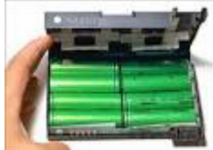
Inside a Laptop Battery
