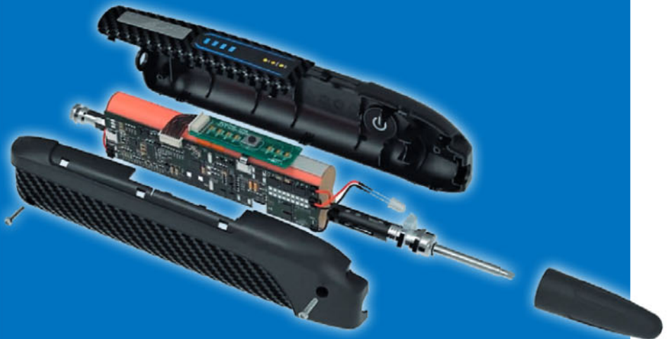
This 3D internal view of the soldering iron showing the battery pack is from the YouTube video: https://youtu.be/8wvwyJlul-0h4 . This same YouTube video also has a 3D external view of the soldering iron.
