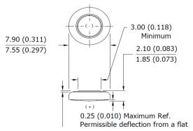
0.06 (0.002) Minimum Ref. (applies to top edge of gasket or edge of crimp, whichever is higher)
