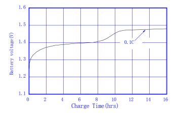
Typical charge curve(at 0.1C  $20\pm5^{\circ}$ C)
