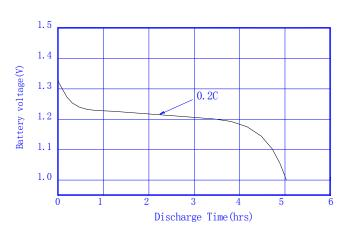
Typical Discharge curve (at  $0.2C\ 20\pm5^{\circ}C$ )
